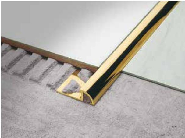
The ROUNDTEC RD profile is mainly used in transitioning floor types of different thicknesses, for example from ceramic tile to thin linoleum. Its rounded section provides a smooth level change of 3mm, making it suitable between two floor types or as an end profile. ROUNDTEC can even be used as stair nosing or edging for tile countertops. Available in brass with patented dovetail anchoring.
